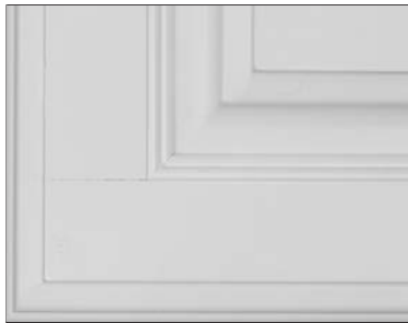
Example of front joint separation
