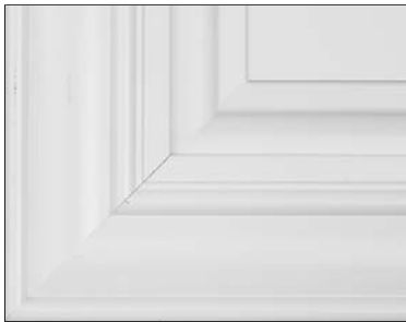
Example of front joint separation
