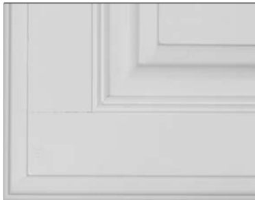
Example of front joint separation
