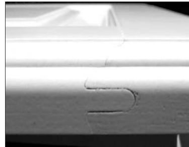
Example of end joint separation
