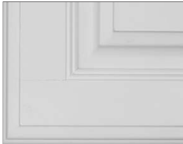
Example of front joint separation
