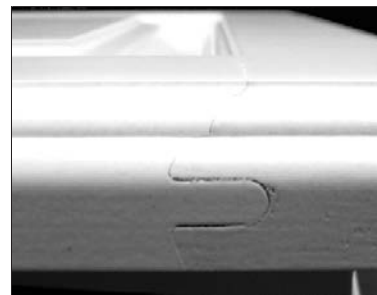
Example of end joint separation
